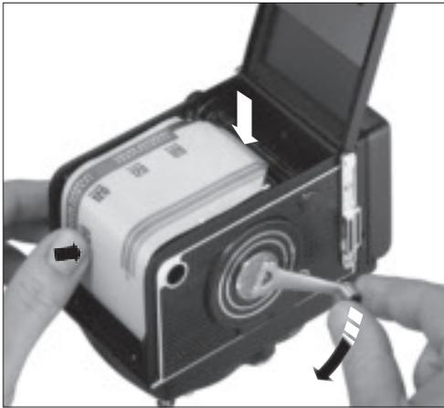
Push the paper leader deeply into the long slot of the empty spool (use the crank 32 for correct positioning). Tighten the film by turning the crank (lower spool must be braked with the thumb) until the arrow sign on the backing paper is in coincidence with the red index on the camera body.
